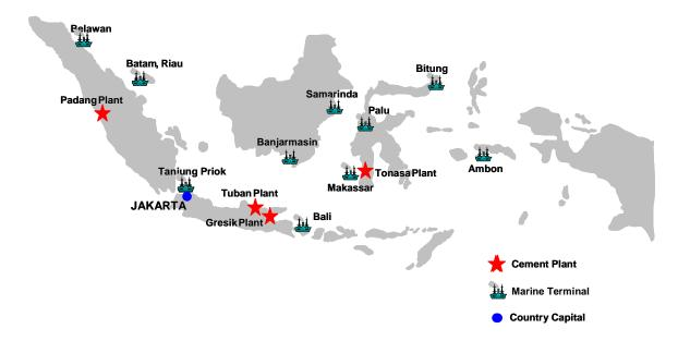
Gresik, with an installed capacity of 17.3 million tons, is Indonesia's largest cement producer. Gresik's production facilities include four plants with twelve dry production lines and one wet production line, with access to most of Indonesia's regions.
