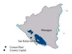
*Description of Properties, Plant and Equipment.* Our Nicaraguan leased cement plant has five kilns utilizing the wet production process with an installed milling capacity of 470,000 tons.
